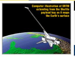
The Shuttle Radar Topography Mission objective is to demonstrate the technology for obtaining high-resolution digital topographic mapping of the Earth. SRTM consists of a specially modified radar system that will fly onboard the space shuttle Endeavour during an 11day mission in early October 1999.
